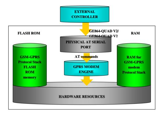
In order to not use any external controller, and further simplify the programming of the sequence of operations, the customer can benefit of these feature already embedded in the modules:
